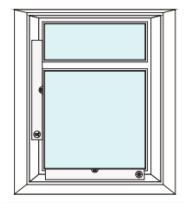
Place the frame at your window and use a spirit level to make sure that it is sitting perfectly straight. For an inside fit frame, you will need to insert packing shims in between the frame and the window so that the frame will stay level and have support. For an inside fit frame we also recommend placing some packers in the corners for extra security against the frame moving and to prevent miters opening up.
